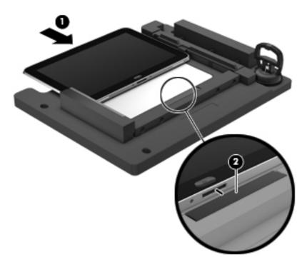
7. Place the suction cup (1) on the lower right corner of the tablet display glass, making sure to place the suction cup inside the edges of the border (2) of the display glass.
